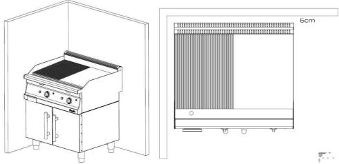
In order for this appliance to be positioned close to a wall, partition, kitchen furniture, decorative covering, etc., the distance between them should be 5 cm, if they are made of non-combustible material or covered with a suitable non- combustible thermal insulation material, otherwise at least 20 cm. It is recommended to pay maximum attention to fire protection rules.
