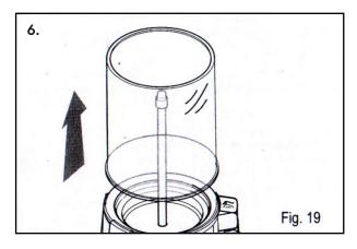
Slide the bowl upwards using both hands. **ATTENTION:** Make sure all liquid is removed from inside the bowl, before removing the bowl.
