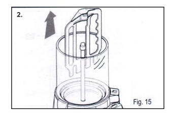
Slide the mixer upwards to remove it. Keep it in line with the central rod until the bottom slot of the mixer itself is level with the rotation pin.
