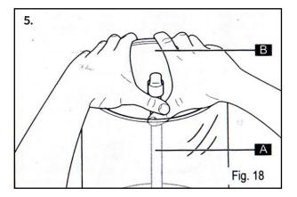
Release the bowl from the machine body. using two fingers to prise it away from the fixed steel part of the mixer auger.
