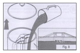
Remove the lid and pour the beverage prepared into the bowl. Never exceed the maximum level which is marked MAX on the bowl itself.
