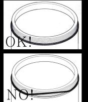
Shown here is the bowl gasket correctly assembled. If the gasket does not perfectly adhere to the bowl edge the liquid will leak out.
