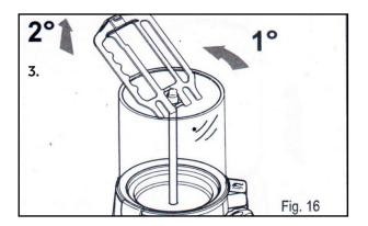
Tilt the mixer over the the mixing auger and slide downwards.
