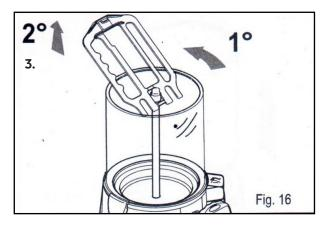
Tilt the mixer and slide it upwards , as illustrated in the figure, to remove it completely.
