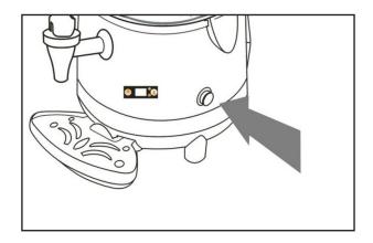
Press the main switch to start the machine. Lit LED = Machine On LED off = Machine Off
