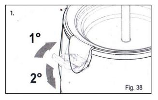
Fix the the bowl to the machine body using the relevant hook-on handles.
