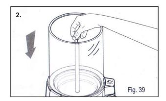
Insert the mixer auger into its seating.
