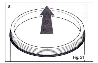
Place the bowl on a flat surface and using both hands, remove the gasket by sliding it upwards in the direction shown by the arrow.
